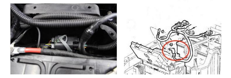
Attach the positive cable to the battery.
