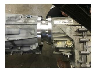
Install the Transfer case shifter bracket using the same nuts that hold the Transfer case onto the adapter (see pic) some light grinding may be needed to clearance the bracket.
