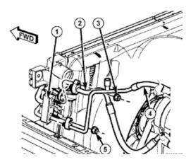
5. Unplug the 34 way Chassis connector (C300) on the lower right hand side of the radiator.
