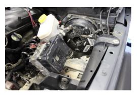
4. Discharge the AC system and remove hoses. Use proper equiptment here guys.
