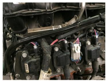
Continue routing the positive alternator to the alternator going along the right side fuel rail and under the throttle body being sure to insulate and secure it.
