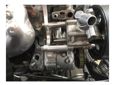
Run the highest heater core port to the return side of the water pump fitting.
