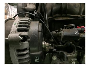
Attach the TIPM positive cable the TIPM (fuse box) stud and secure.
