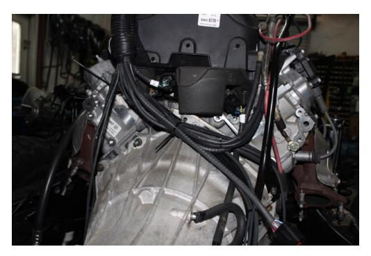
We usually fab up a heat shield or heat wrap the fuel and purge line as it passes from the fuel tank to the transmission. It would also be advisable to fabricate a heat shield for both catalytic converters.
