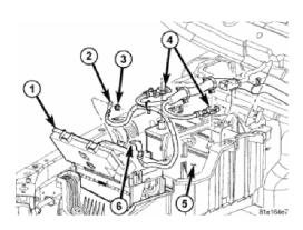
Disconnect the steering shaft at the firewall.
