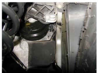
Run harness around the brake booster and plug into the two 14 way connectors on the main under hood harness.
