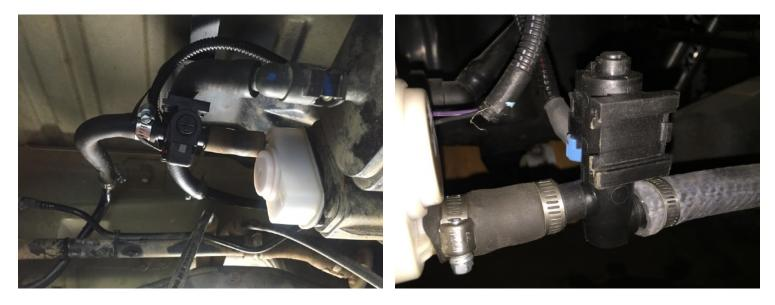
IF YOU PLAN ON MOVING YOUR EVAP CANISTER NOW IS A GOOD TIME. JUST KEEP ALL THE HOSES RUNNING TO THE SAME PORTS AND YOU WILL BE FINE. WE USUALLY MOVE THE CANISTER TO THE RIGHT REAR SPRING PERCH AREA.
