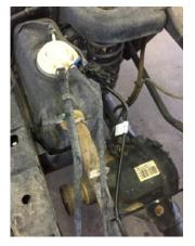
CUT THE LARGE HOSE THAT RUNS BETWEEN THE FILLER NECK AND THE CANISTER CLOSE TO THE WHITE VALVE. ATTACHED GM VENT VALVE INLINE WITH THIS HOSE AND SECURE WITH HOSE CLAMPS. PLUG INTO THE NEW HARNESS AND SECURE.
