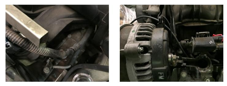
Attach the TIPM positive cable the TIPM (fuse box) stud and secure.
