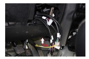
Locate the three white connectors labeled x101, x102 and x103. Plug these into the EZcanbus Module matching the positions on the labels. Mount the module under steering column or along the inner fender area making sure the harness does not rub the steering shaft. We like to keep it as high as possible just in case you get into high water.
