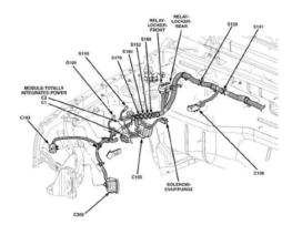
6. Unplug the Jeep computer connectors C1 C2 and C4 for 07-11 and C2 for 12+. One harness will stay with the body and the rest will go with the engine.
