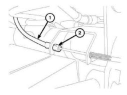
18. Disconnect the transmission and transfer case cables. #2 and #3 pictured below
