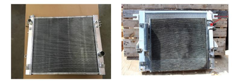
Assemble the fan and AC condenser to the radiator using original hardware. Be sure to reuse the rubber flaps on the sides.
