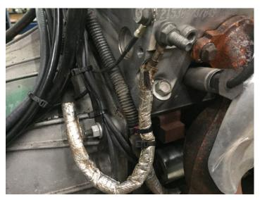
Route both wires up and over the starter to the rear of the engine and up the RH rear cylinder head. Be sure to insulate and secure the wires away from heat.
