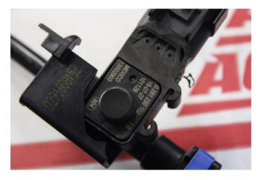
For 07-11 install the new fuel tank pipe sensor hose in place of your original one.
