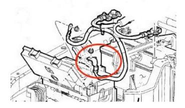
Attach the positive cable to the battery.
