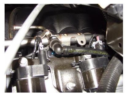
We usually start off with the engine installed and the body off. If you're doing the swap with the body on it will be a little more difficult but can be done. You want to be very careful not to route the line near the exhaust system or anything sharp.
