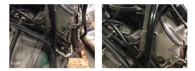
Continue running up the RH fuel injector rail and branch off the cables to the battery and TIPM.
