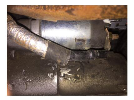
Attach the main ground wire to the engine block or rear cylinder head. You probably don't want to use a stud to attach even though we did in this picture.
