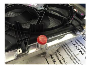
The fan shroud will slide into the lower tabs on the radiator and secure at the top with the original hardware. It may be necessary to clearance the plastic around the upper or lower radiator hose to allow room for the hose clamps.
