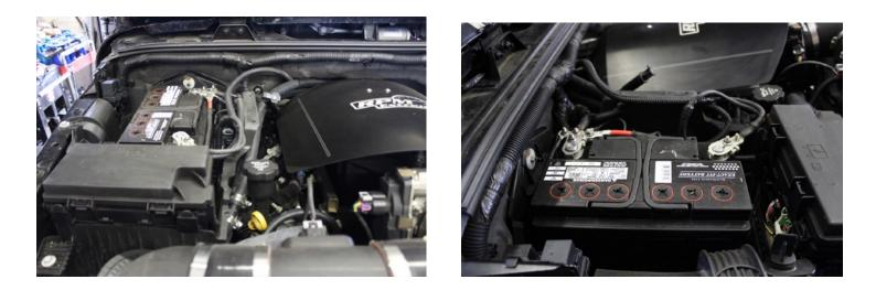
TECH TIP: Always remove the negative cable from the battery first and install it last. This will prevent arcing and will protect the computers and electronics.
