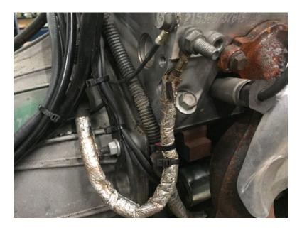
Route both wires up and over the starter to the rear of the engine and up the RH rear cylinder head. Be sure to insulate and secure the wires away from heat.
