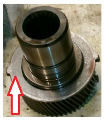
Take your new input shaft and transfer the index washer over to it. Place the new input shaft into the synchronizer aligning the tabs on the index washer. Install the snap ring and be sure its seated into the grove.
