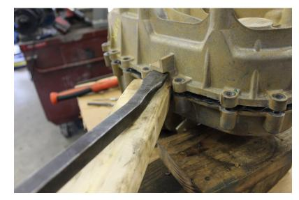
Carefully remove the top case and set aside. You will now see the chain and gears
