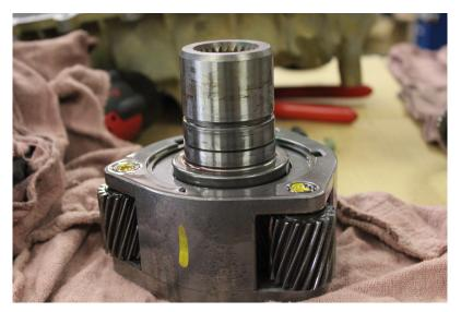
With the synchronizer removed locate and remove the snap ring on the input shaft side. Then remove the input shaft and index washer.
