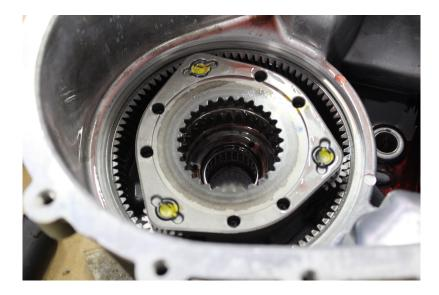
Lay the case on its side and use a soft hammer to tap the input shaft towards the inside of the case. The input shaftplanetary assembly should come out as an assembly. CAUTION.... You did remove the seal and snap ring before you split the case correct?
