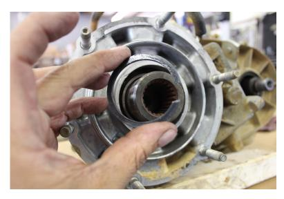
Flip the case over so the input is down.
