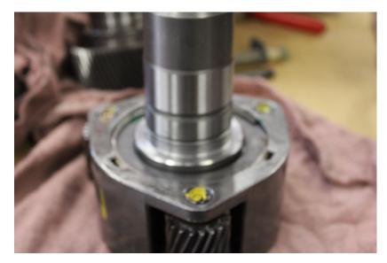
Insert the synchronizer assembly back into the housing and install the snap ring on the front side of the input shaft. Then install the seal being careful not to crush or damage it.
